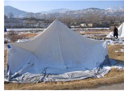
Archive photo – tent failure under snow load due to guy lines pulling out, Allai. (source Jos Miesen / IFRC)
