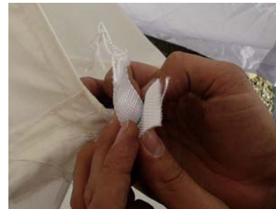
Detail of white webbing that has pulled through.
