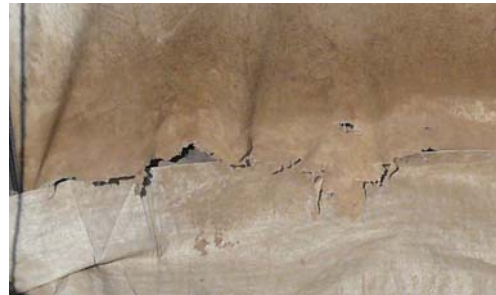
Decayed canvas due to short mud flaps, Jaba Camp.
