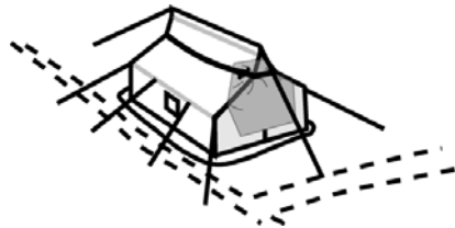
blanket or plastic sheeting covering unused door. note drainage ditches and site drainage around tent
